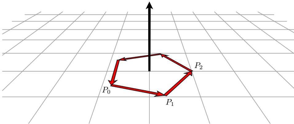
**normal function:2** Associated to an oriented polygon in 3D is what I call its **normal function**, the unique linear function  $Ax + By + Cz + D$  with these three properties:
