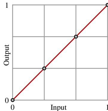
For an arbitrary straight line fudge function, choose the values in the array so that  $(0, s_0)$ ,  $(1/3, s_1)$ ,  $(2/3, s_2)$ ,  $(1, s_3)$  all lie in a straight line.
