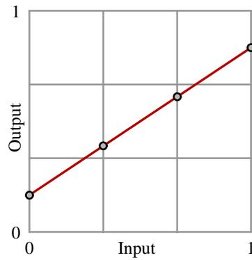
For non-linear fudging, the control values  $s_1$  and  $s_2$  are chosen to force the fudge graph to lie close to the points  $(1/3, s_1)$  and  $(2/3, s_2)$  without passing through them. There is a fault with this scheme, since the amount of contrast it can achieve is limited:
