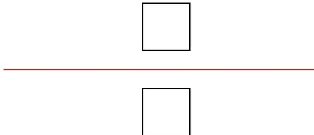
In other words, we divide space into two parts by a plane. Each side of this plane contains one of the cubes. The question of nearest and farthest is determined by determining which side of this plain the eye (or, in practice, what I have called the **virtual eye**) is on.
