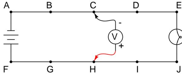
Using a voltmeter, a technician measures 0 volts between the points C and H. The result of this single measurement indicates which half of the circuit there is a definite problem in. What would you recommend as the *next* voltmeter measurement to take in troubleshooting the circuit, following the same "divide in half" strategy?
