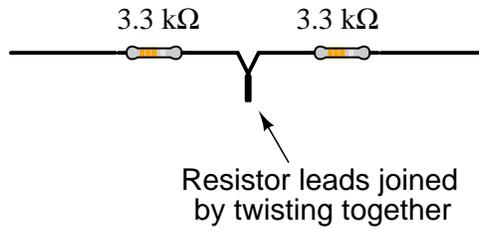
How much electrical resistance would you expect an ohmmeter to indicate if it were connected across the combination of these two series-connected resistors?
