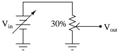
Describe the mathematical relationship between  $V_{in}$  and  $V_{out}$  with the potentiometer in this position. What does this suggest about the usefulness of a potentiometer as an analog computational element?
