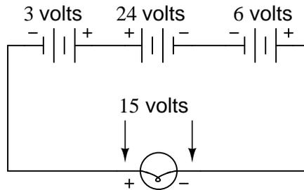
Follow-up question: being that 30 volts is the commonly accepted "danger" threshold voltage for electric shock, determine whether or not this particular circuit poses a shock hazard.
