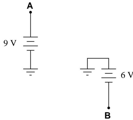
The student has already figured out that  $V_A = +9 \text{ V}$  and  $V_B = -6 \text{ V}$ , but does not know for certain how to calculate the voltage between points **A** and **B**. Asking her instructor for an explanation, the instructor begins to draw this illustration:
