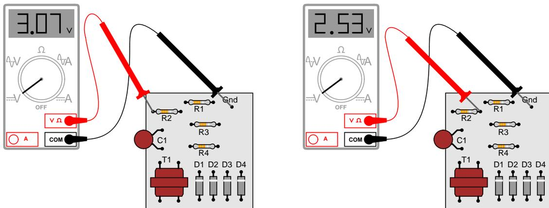
R2's color code is Orange, Orange, Red, Gold. Based on this information, determine both the direction and the magnitude of DC current through resistor R2, and explain how you did so.
