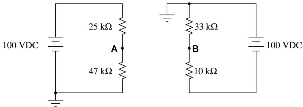
Now, calculate the voltage between points **A** and **B** ( $V_{AB}$ ).
