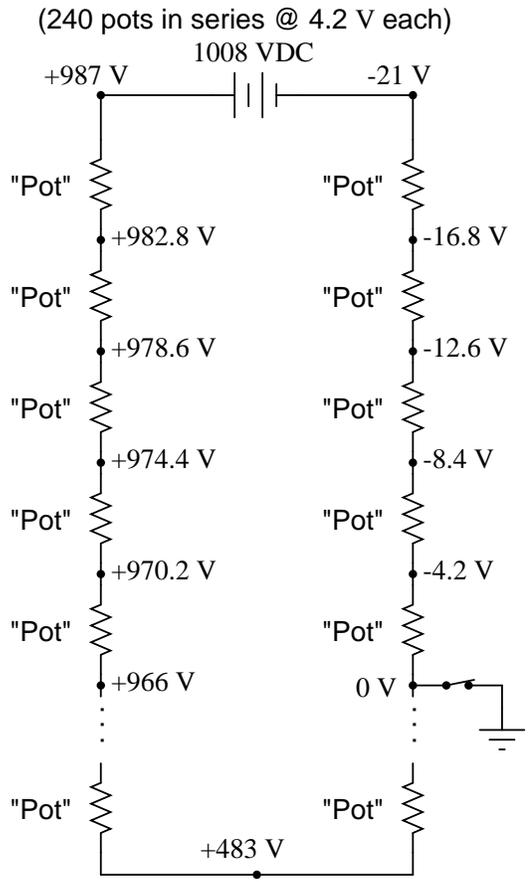
Determine the voltages (with respect to earth ground) for each of the points (dots) in the following schematic diagram, for the ground location shown:
