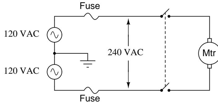
One day the motor suddenly stops running, even though the switch is still in the "on" position. An electrician is summoned to troubleshoot the failed motor, and this person decides to perform some voltage measurements to determine whether or not one of the fuses has "blown" open before doing anything else. The measurements taken by the electrician are as such (with the switch in the "on" position):
