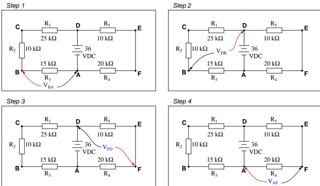
How much voltage would be registered by the voltmeter in each of the steps? Be sure to include the sign of the DC voltage measured (note the coloring of the voltmeter leads, with the red lead always on the first point denoted in the subscript:  $V_{BA}$  = red lead on "B" and black lead on "A"):
