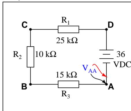
How much voltage would be registered by the voltmeter in each of the steps? Be sure to include the sign of the DC voltage measured (note the coloring of the voltmeter leads, with the red lead always on the first point denoted in the subscript:  $V_{BA}$  = red lead on "B" and black lead on "A"):
