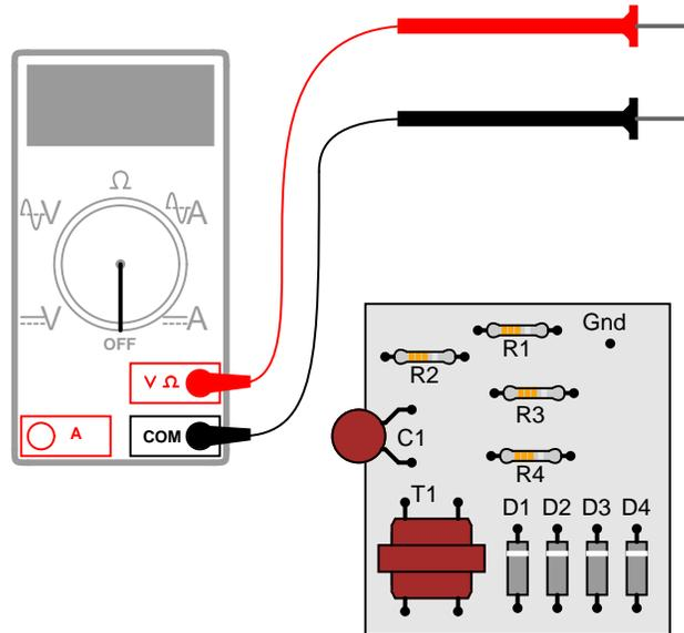
So, you decide to touch the black probe of the voltmeter to the circuit's "Gnd" (ground) test point, and measure the voltage with reference to ground on both sides of R2. The results are shown here:
