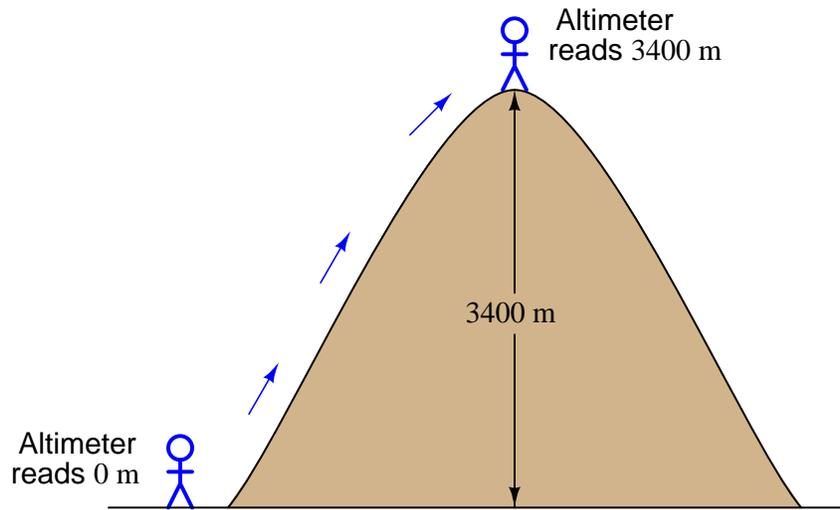
While at the summit, the climber may re-set the altimeter's "zero" adjustment to register 0 meters once again. If the climber then descends to the base of the mountain, the altimeter will register -3400 meters:
