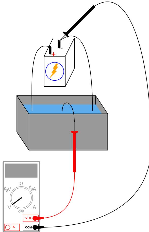
Which way would you have to move the middle wire (the one touching the voltmeter's red test lead) in order to increase the voltmeter's reading?
