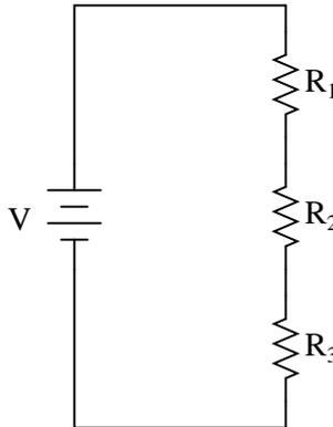
$$I = f(V, R_1, R_2, R_3)$$
