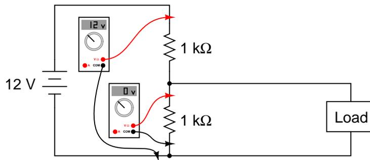
Based on these measurements, the technician concludes that the upper resistor must be failed open. Upon disassembling the divider circuit and checking resistance with an ohmmeter, though, both resistors are revealed to be in perfect operating condition.
