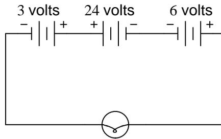
Also, identify the polarity of the voltage across the light bulb (mark with "+" and "-" signs).
