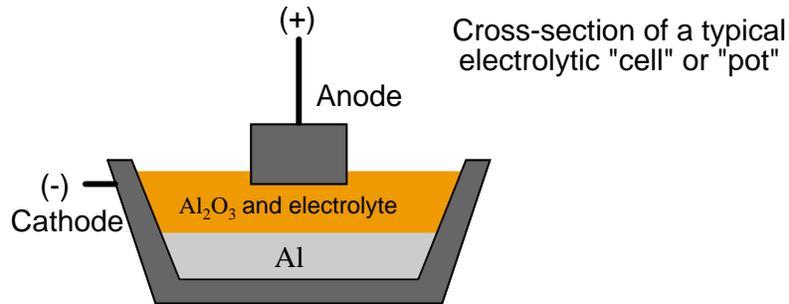
The alumina/electrolyte mixture is a molten bath of chemicals, lighter than pure aluminum itself. Molecules of pure aluminum precipitate out of this mix and settle at the bottom of the "pot" where the molten metal is periodically pumped out for further refining and processing. Fresh alumina powder is periodically dropped into the top of the pot to replenish what is converted into aluminum metal.
