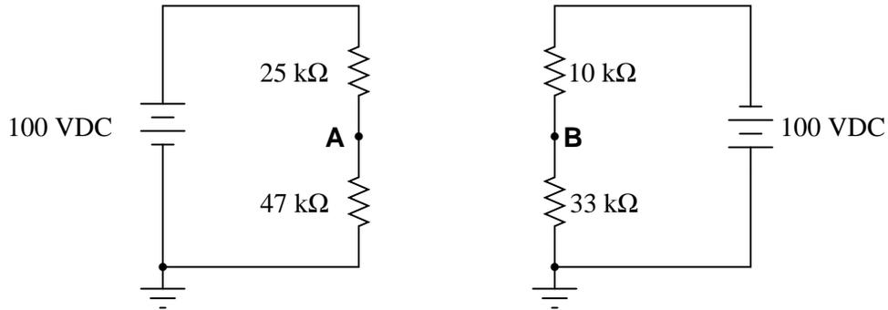
To make it even easier to visualize, remove the ground symbols and insert a wire connecting the lower wires of each circuit together:
