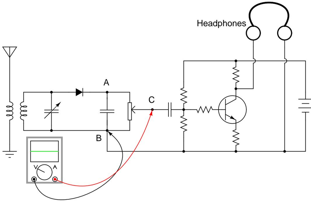
What do these voltage measurements indicate about the nature of the problem in the receiver circuit?
