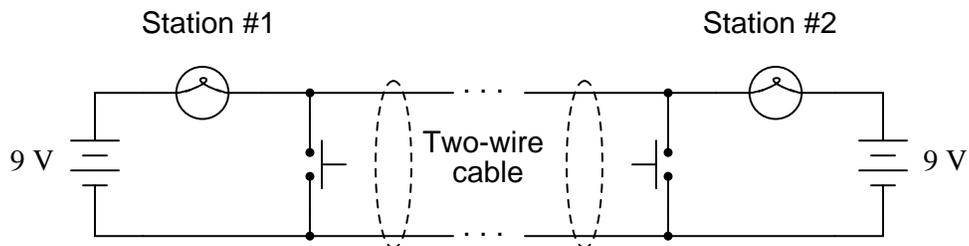
Explain why the lamps energize when either pushbutton is actuated, and why they de-energize when both pushbuttons are open (despite there being an unbroken circuit connecting both lamps and both batteries).
