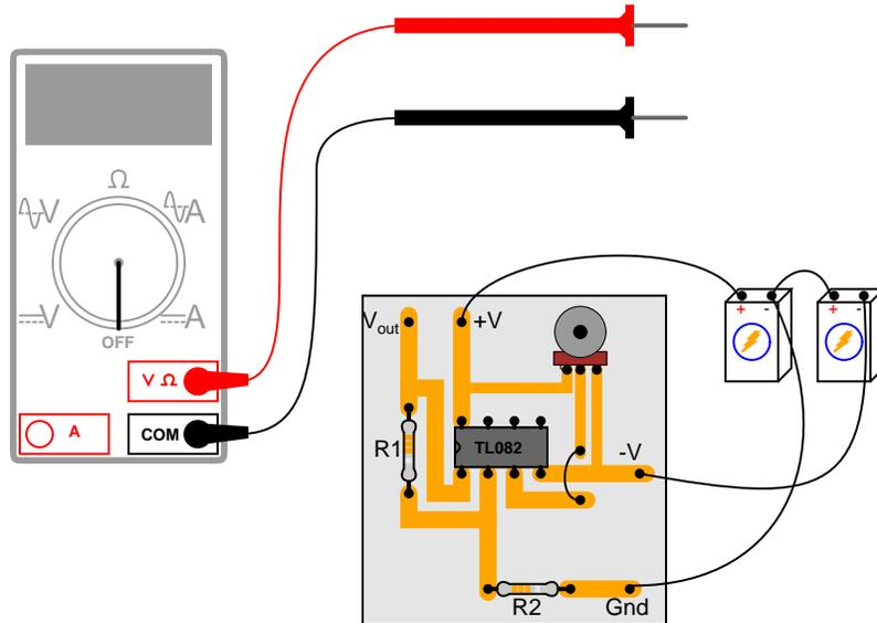
She decides to measure the voltage on either side of resistor R1 with reference to ground, and obtains these readings:
