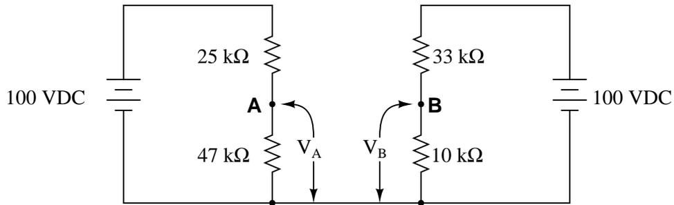
Now, calculate the voltage between points **A** (red lead) and **B** (black lead) ( $V_{AB}$ ).
