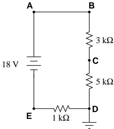
For example,  $V_B$  means the voltage indicated by a voltmeter with the red test lead touching point B and the black test lead touching ground.
