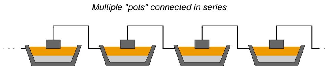
A typical "pot-line" might have 240 pots connected in series. With a voltage drop of just over 4 volts apiece, the total voltage powering this huge series circuit averages around 1000 volts DC:
