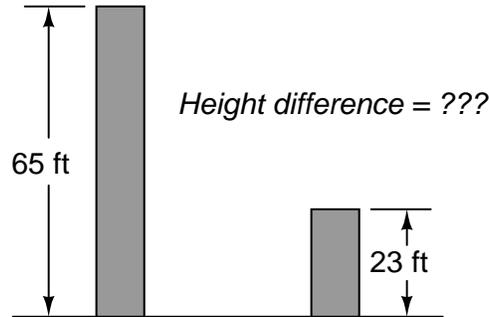
The height of each object is analogous to the voltage dropped across each of the lower resistors in the voltage divider circuits. Like voltage, height is a quantity measured *between two points* (the top of the object and ground level). Also like the voltage  $V_{AB}$ , the difference in height between the two objects is a measurement taken between two points, and it is also found by subtraction.
