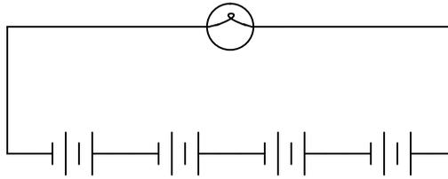
Follow-up question: if each of these batteries outputs a voltage of 1.5 volts, how much voltage does the light bulb experience?
