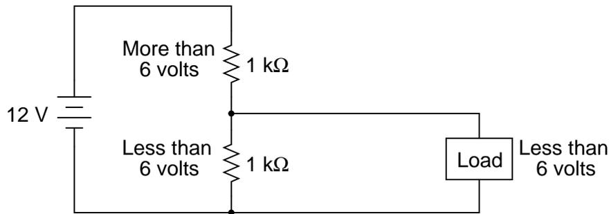
(Of course, with no load connected, the voltage across the lower resistor would be precisely 6 volts. With the load connected, the parallel combination of load and 1 kΩ resistor results in an effective resistance of less than 1 kΩ on the lower half of the divider, resulting in a voltage of less than half the total supply voltage.)
