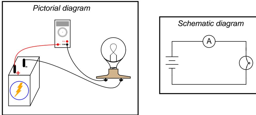
In order to practically function, an ammeter must have some internal resistance. It is usually a very small amount, but it does exist. It should be apparent to you that the presence of this resistance will have some effect on the circuit current, when compared to the amount of current in the circuit without any meter connected:
