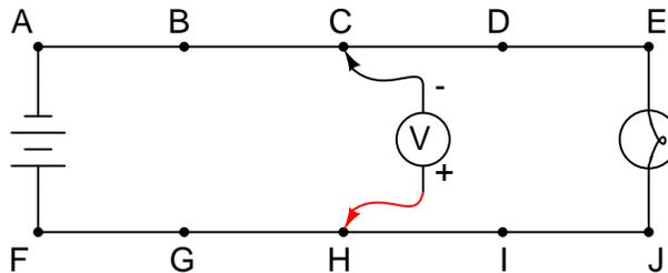
Using a voltmeter, a technician measures 0 volts between the points C and H. What does this single measurement indicate about the condition of the circuit? Be as specific as you can.
