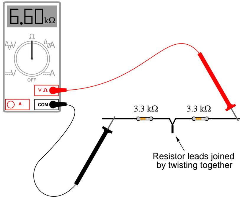
Follow-up question: how much resistance would you expect the ohmmeter to register if there were *three* similarly-sized resistors connected in series instead of two? What if there were *four* resistors?
