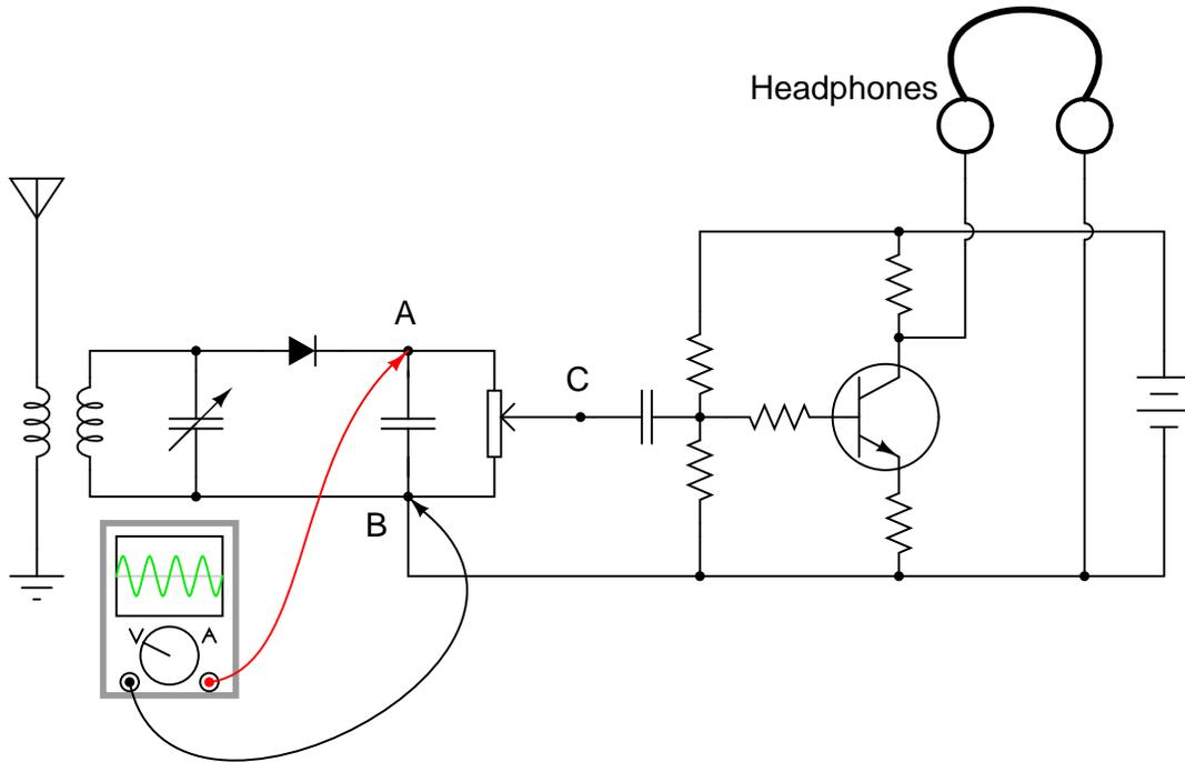
However, when checking between points C and B in the circuit, no signal is measured:
