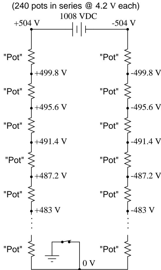
Follow-up question: assuming each of the pots acts exactly like a large resistor (which is not entirely true, incidentally), what is the resistance of each pot if the total "potline" current is 150 kA at 4.2 volts drop per pot?
