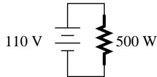
Now suppose that exact same heater is connected to one end of a long two-wire cable, which is then connected to the same 110 volt source. Assuming that each conductor within the cable has an end-to-end resistance of 3 ohms, how much power will the heater dissipate?
