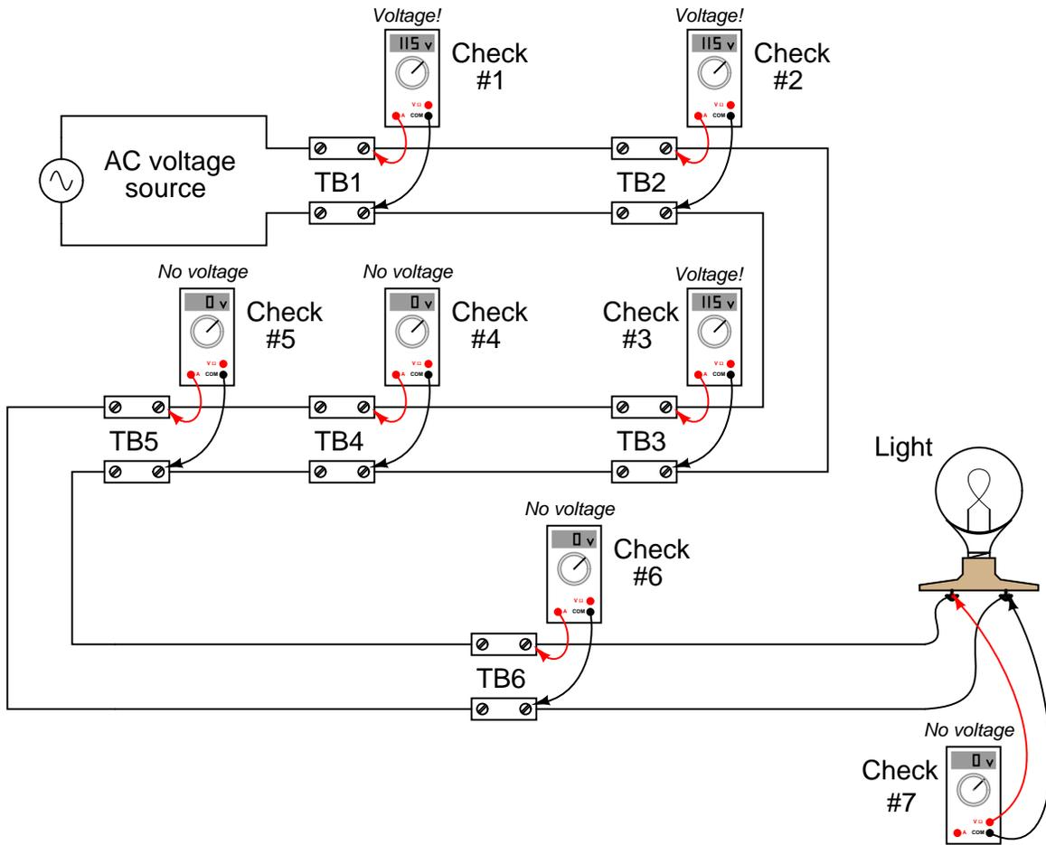
Based on the voltage indications shown, can you determine the location of the circuit fault? What about the electrician's choice of steps – do you think the voltage measurements taken were performed in the most efficient sequence, or would you recommend a different order to save time?
