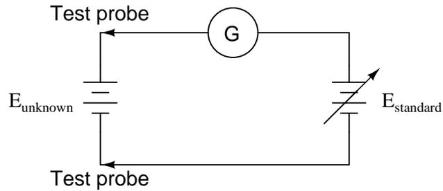
The technique is to adjust the standard voltage source until the galvanometer registers exactly zero. When this condition is met, the system is said to be "balanced," indicating that the two voltage sources are equal in magnitude to each other. This voltage magnitude is then read from the calibrated adjustment dial on the standard source.
