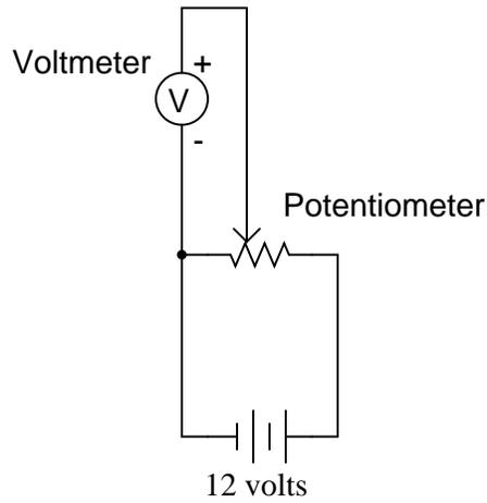
What would you expect the voltmeter to register if the wiper were set precisely at the 50% (half-way) position?
