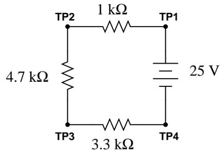
$$V_{TP1-TP3} = \quad V_{TP2-TP4} =$$
