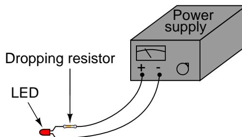
Calculate the necessary resistance value and minimum power rating of a series dropping resistor for an LED rated at 1.7 volts and 20 mA, and a power supply voltage of 24 volts.
