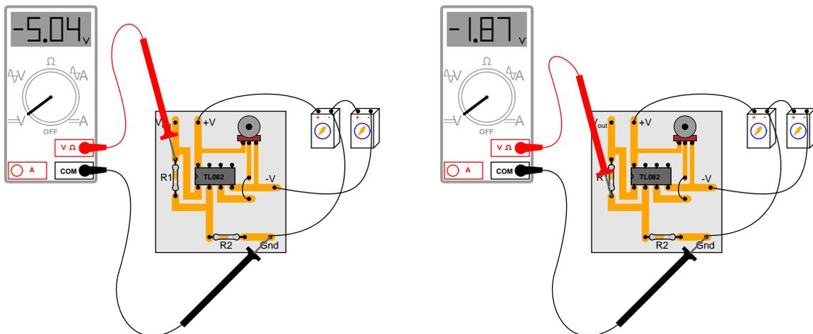
On the top side of R1, the voltage with reference to ground is -5.04 volts. On the bottom side of R1, the voltage with reference to ground is -1.87 volts. The color code of resistor R1 is Yellow, Violet, Orange, Gold. From this information, determine the following:
