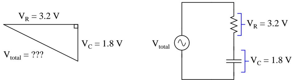
Explain what equation(s) you use to calculate  $V_{\text{total}}$ , as well as why we must geometrically add these voltages together.
