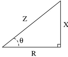
Suppose we wished to know the value of angle  $\Theta$ , and we happened to know the values of  $Z$  and  $R$  in this impedance triangle. We could write the following equation, but in its present form we could not solve for  $\Theta$ :
