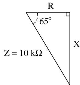
We know that the *sine* function relates the sides  $X$  and  $Z$  of this impedance triangle with the  $65$  degree angle, because the sine of an angle is the ratio of *opposite* to *hypotenuse*, with  $X$  being opposite the  $65$  degree angle. Therefore, we know we can set up the following equation relating these quantities together:
