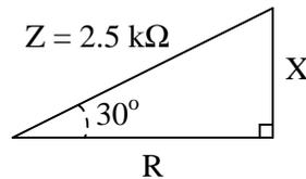
Use the appropriate trigonometric functions to calculate the equivalent values of  $R$  and  $X$  in this series circuit.
