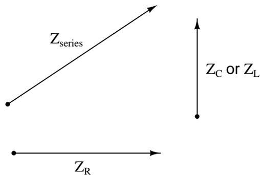
Since the phasor for resistive impedance ( $Z_R$ ) has an angle of zero degrees and the phasor for reactive impedance ( $Z_C$  or  $Z_L$ ) either has an angle of +90 or -90 degrees, the *phasor sum* representing total series impedance will form the hypotenuse of a right triangle when the first two phasors are added (tip-to-tail).
