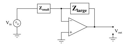
This opamp circuit has the greater voltage gain, because its  $\frac{Z_{feedback}}{Z_{input}}$  ratio is greater.
