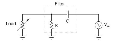
In this active filter circuit, how will the filter's cutoff frequency be affected by changes in the load resistance? Be as specific as you can in your answer.
