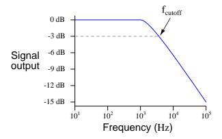
What does the term *rolloff* refer to, in the context of filter circuits and Bode plots? Why would this parameter be important to a technician or engineer?
