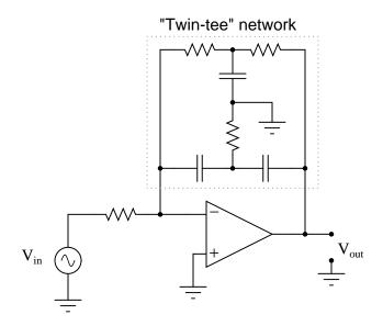
Identify which of these circuits is band-pass, and which is band-stop. Also, identify the type of response typically provided by the twin-tee network alone, and how that response is exploited to make two different types of active filter responses.
