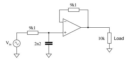
Determine the type (LP, HP, BP, BS) and cutoff frequency of this active filter circuit:
