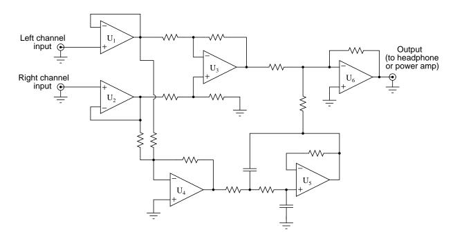
The circuit works on the principle that vocal tracks are usually recorded through a single microphone at the recording studio, and thus are represented equally on each channel of a stereo sound system. This circuit effectively eliminates the vocal track from the song, leaving only the music to be heard through the headphone or speaker.
