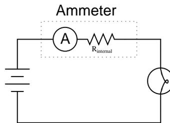
Explain why it is usually safe to ignore the internal resistance of an ammeter, though, when it is in a circuit. A common term used in electrical engineering to describe this intentional oversight is *swamping*. In this particular circuit an engineer would say, "The resistance of the light bulb *swamps* the internal resistance of the ammeter."
