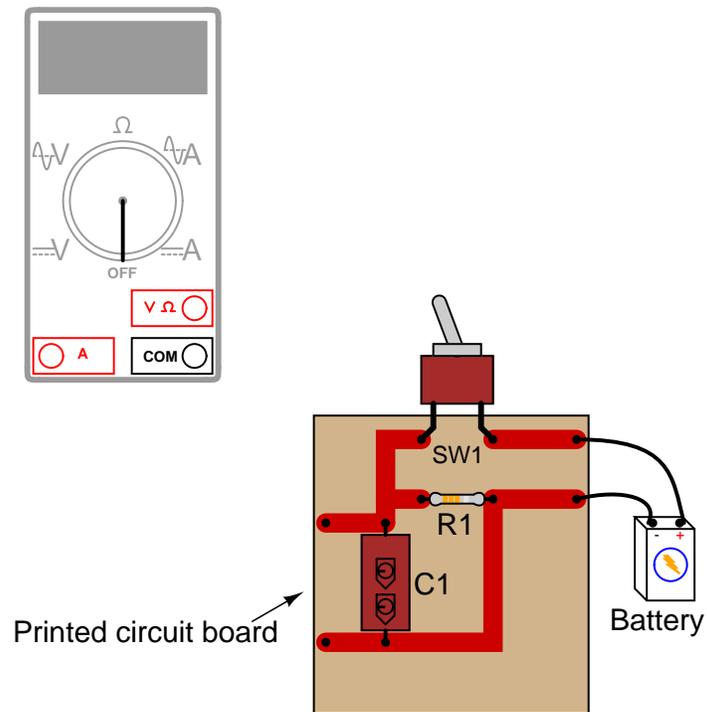
How would the multimeter be used to measure the current through the component labeled "R1" when energized? Include these important points in your answer:
