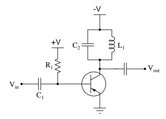
This circuit will look very strange if you are accustomed to analyzing audio-frequency and DC amplifier circuits. Note some of the distinct differences between this amplifier and an amplifier used to boost audio signals. Also, explain what "class-C" operation means, and how this amplifier is able to output a continuous sine wave despite the transistor's behavior in class-C mode.
