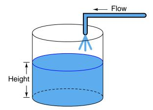
In calculus terms, we would say that the tank *integrates* water flow into water height. That is, one quantity (flow) dictates the rate-of-change over time of another quantity (height).
