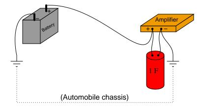
What is the purpose of having a capacitor connected in parallel with the amplifier's power terminals? What benefit does this give to the audio system, overall?
