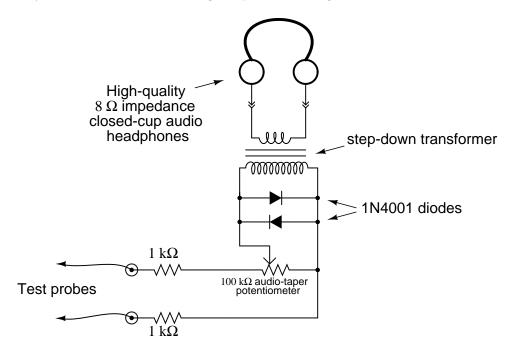
What purpose do the two diodes serve in this circuit? Hint: if you remove the diodes from the circuit, you will not be able to hear the difference in most cases!
