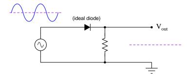
Sketch the shape of the output voltage waveform for this "clipper" circuit, assuming an ideal diode with no forward voltage drop:
