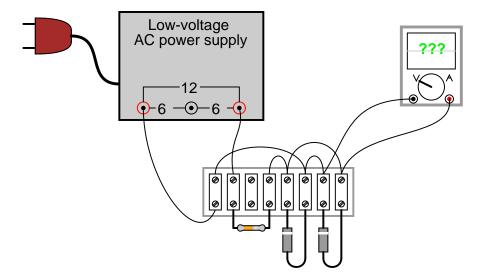
The diodes are model 1N4001, each. The resistor's color code is Brown, Black, Orange, Silver.  $\underline{\text{file }01108}$
