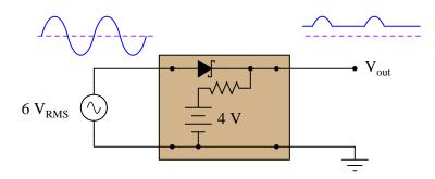
Follow-up question: explain why a *Schottky* diode is shown in this circuit rather than a regular silicon PN-junction diode. What characteristic(s) of Schottky diodes make them well suited for many clipper applications?
