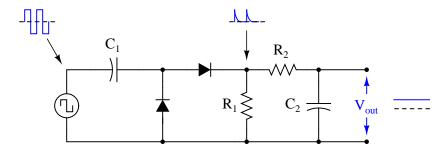
Explain what happens to the output voltage as the input frequency is increased, assuming the input voltage amplitude does not change. Can you think of any practical applications for a circuit such as this?  $\underline{\text{file }02129}$
