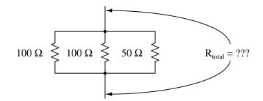
No, this is not a "trick" question! There is a way to apply a two-resistance equation to solve for three resistances connected in parallel.
