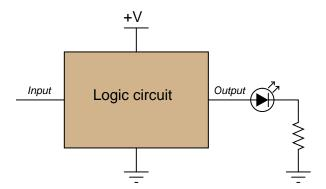
Complete this schematic diagram by including a switch in the drawing, such that in each of its two positions, a definite "low" or "high" logic state will be sensed by the circuit's input terminal.
