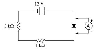
Usually, ammeters are connected in *series* with the component whose current is to be measured. However, in this case a parallel connection is acceptable. Explain why, and determine the ammeter's current reading in this circuit.
