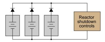
Challenge question: it would be nice if there were indicator lamps in the system to warn maintenance personnel of a shorted power supply. Is there any way you can think of to place light bulbs in this system somewhere, so that one will light up in the event of a power supply failure?
