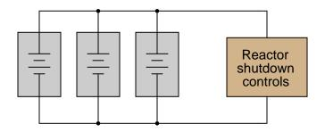
The only problem with this scenario is the possibility of one of these power sources internally short-circuiting. Describe what would happen if one of the three DC power sources developed an internal short-circuit, and explain how this problem could be avoided by placing diodes in the circuit.
