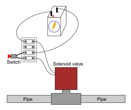
The only problem with this simple circuit is that the switch contacts suffer from extensive arcing caused each time the solenoid is de-energized. One way to combat this arcing, though, is to connect an ordinary rectifying diode in parallel with the solenoid like this:
