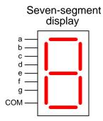
A special decoder circuit is needed to translate 4-bit BCD codes into the particular combinations of segment activations that represent decimal digits.
