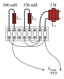
Also, write a formula that calculates total inductance given the values of inductors  $L_1$ ,  $L_2$ , and  $L_3$ . file 00379
