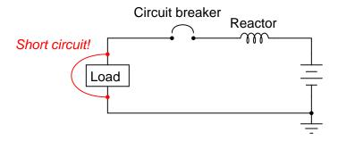
Explain how the addition of a "reactor" helps to minimize the magnitude of the short-circuit current the breaker has to interrupt.
