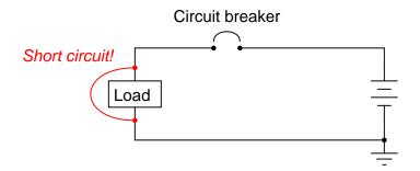
The purpose of the circuit breaker, of course, is to open the circuit automatically, to prevent damage to the power conductors. In a large electric power system, the magnitudes of such short-circuit currents can be enormous.
