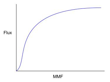
What does this graph indicate to you, as compared to the graph for a resistor's characteristics? What is the significance of this with regard to magnetic "circuit" analysis?  $\frac{\text{file }00682}{\text{file }00682}$
