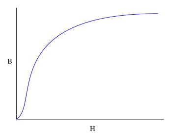
Rarely will you see a plot of flux  $(\Phi)$  shown as as a function of MMF  $(\mathcal{F})$ , even though such a plot would appear very similar to the "B/H curve" for that same material. Why is this? Why would a "B/H" curve be preferable to an engineer rather than a "Flux/MMF" curve?
