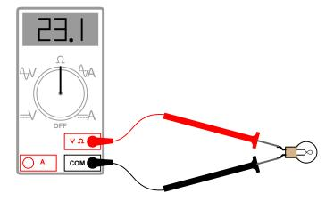
Also, identify the reading you would expect the ohmmeter to indicate if the light bulb were burnt out (failed "open").
