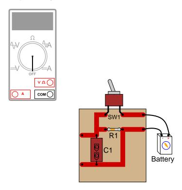
How would the multimeter be used to measure the resistance of the component labeled "R1"? Include these important points in your answer:
