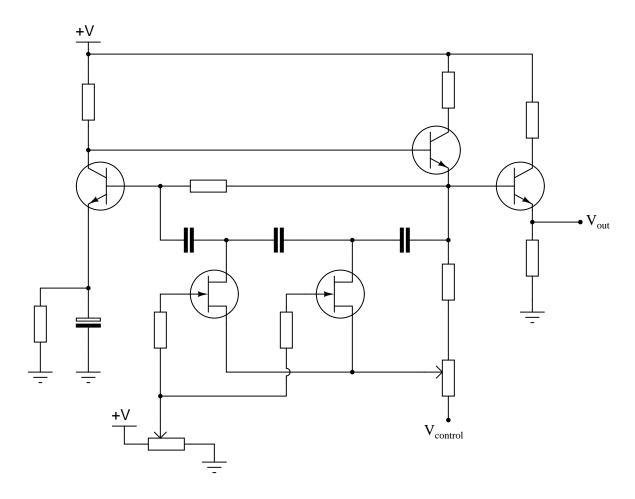
The oscillator is of the RC "phase shift" design. Explain how this circuit works. Why does the output frequency vary as the control voltage varies? Does the output frequency increase or decrease as the control voltage input receives a more positive voltage?
