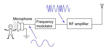
This is how FM radio communication works: by modulating the frequency of a radio-frequency (RF) signal according to the amplitude of the voltage signal produced by a microphone.
