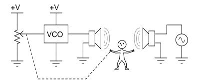
If a voltmeter were connected between the potentiometer wiper and ground, what would its indication represent (with regard to the external audio signal)?
