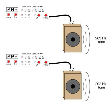
Explain how this phenomenon could be used by a technician to adjust two audio frequency sources to the same frequency, without the aid of any expensive test equipment such as a frequency counter or an oscilloscope.
