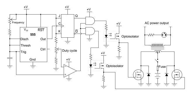
Please note that this is only a general schematic, and may not be exactly what you need to build in order to have a successful inverter circuit. Your choice of specific power components (transformer, power MOSFETs, zener diodes) are critical. Paralleled MOSFETs and zener diodes may very well be in order!
