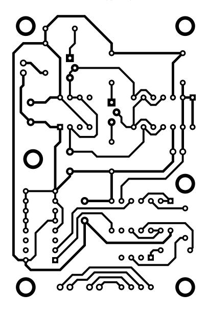
Mark where discrete components (resistors, capacitors, and diodes) go into the PCB, and identify which integrated circuits on the board layout are performing which functions in the schematic. Note: the square pad on each IC marks pin number 1.
