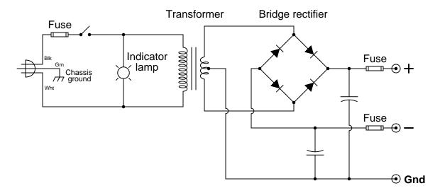
Of course, you are not restricted to using this exact design. One design feature I insist on, though, is that you build your own rectifier circuit from individual diodes, rather than use a packaged rectifier assembly. I highly recommend the use of "barrier strips" or "terminal strips" to make the electrical connections between components. These connection devices provide solid, permanent electrical connections while still allowing components to be easily installed and removed.
