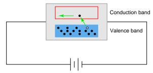
With sufficient thermal energy, these electron-hole pairs will form spontaneously. At room temperature, however, this activity is slight.
