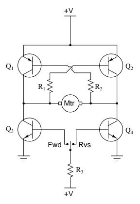
At any given moment, how many transistors are turned on and how many are turned off? Also, explain what would happen to the function of the circuit if resistor R1 failed open.  $\frac{\text{file }00449}{\text{constant}}$
