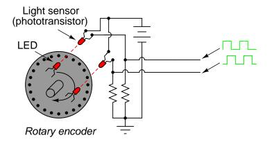
The two LED/phototransistor pairs are arranged in such a way that their pulse outputs are always  $90^{\circ}$  out of phase with each other. Quadrature output encoders are useful because they allow us to determine direction of motion as well as incremental position.
