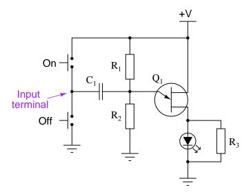
Explain how the unijunction transistor functions in this circuit.  $\underline{{\rm file}~01128}$
