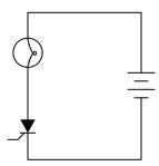
Next, explain what must be done to turn the SCR off so that the light bulb de-energizes.  $\underline{\text{file }02136}$
