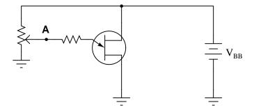
Now describe what must be done to the potentiometer to cause the UJT to turn back off again.  $\underline{\text{file }02144}$
