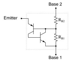
When the two base terminals of a UJT are connected across a source of DC voltage, the two base resistances ( $R_{B1}$  and  $R_{B2}$ ) form a voltage divider, splitting the applied voltage into lesser portions:
