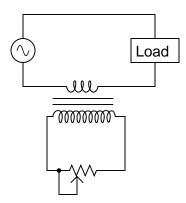
Calculate the amount of series impedance the transformer places in the load current's path, if the variable resistor is set to a resistance of 15 ohms, and the winding ratio is 20:1.
