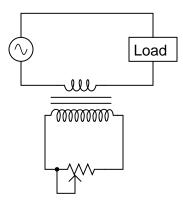
With this circuit, power to the AC load may be controlled by the variable resistor's setting:
