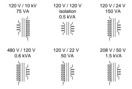
Design a circuit that uses one or more of these transformers to reduce the line voltage (120 VAC) down to an appropriate level so that the 600 watt heater will only output (approximately) 400 watts.  $\frac{\text{file }00094}{\text{email}}$
