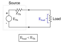
In this diagram, the source's internal impedance has been "lumped" into a single component, labeled  $Z_{Th}$ , the Thévenin impedance. This intrinsic impedance naturally limits the amount of power any source can deliver to a load. It also creates a condition where load power is optimized at a particular load impedance.
