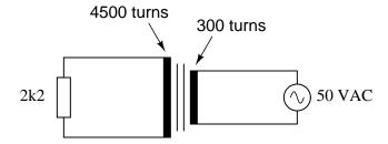
Calculate the amount of power supplied by the source in each of these circuits:
