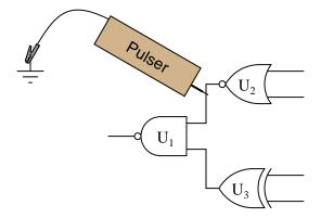
Which gate, or gates, are we testing by placing the pulser in this position? What other instrument(s) would we have to connect to the circuit (and where?) to complete the test? Why does the logic pulser require a ground connection to do its job in this circuit?
