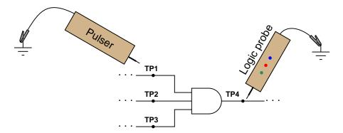
No matter which input test point (TP1, TP2, or TP3) she pulses, though, the output test point (TP4) always reads low. Does this prove the AND gate to be defective? Explain why or why not. file 03840
