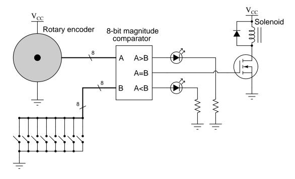
Trace the directions of all currents in this circuit, using electron flow notation, when the encoder position matches the pre-set code entered at the switches. Then, identify specific component failures that could result in the solenoid coil not energizing in this condition.
