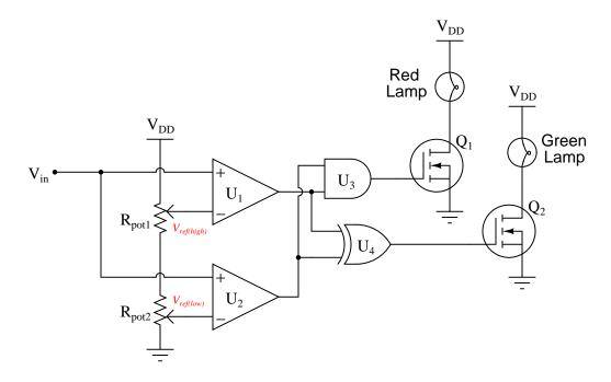
A technician decides to replace the red lamp, thinking it is burned out. This, unfortunately, does not fix the problem. Identify two possible component faults that could account for this problem, and describe what further diagnostic steps you would take to determine the precise nature of the fault.
