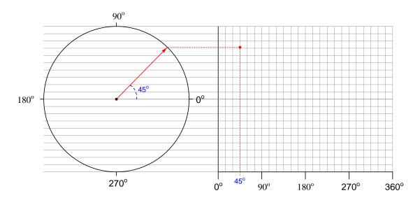
You may wish to use a *protractor* to precisely mark the angles along the rotation of the circle, in making your sine-wave plot.
